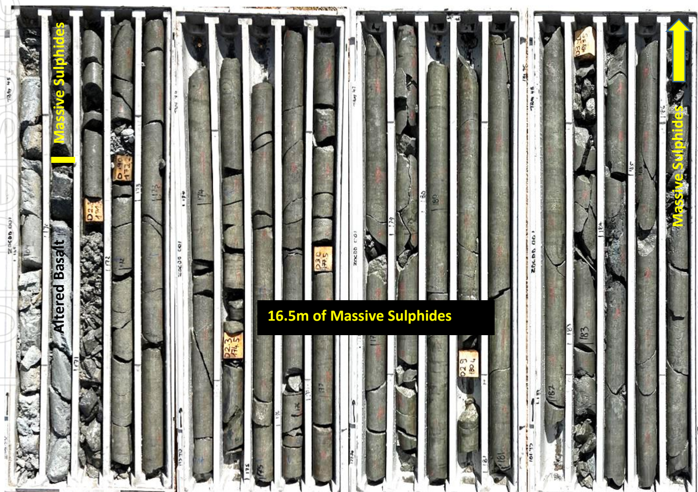
Figure 1: Photograph of 16.5m of Copper-Zinc-Iron Massive Sulphides (170.4m to 186.9m) in Zenith Diamond Hole ZDCDD001 Develin Creek Copper-Zinc Project – QLD (4 core trays approx. 4.5m per tray)
